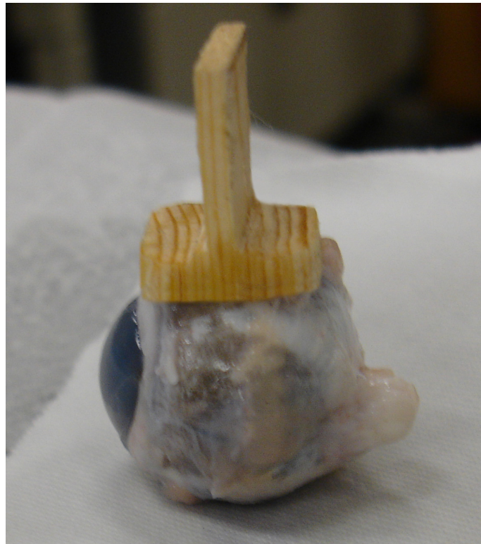
Figure 20. The T-structure adhered to the porcine sclera prior to placing into the vacuum eye holder. The bonding surface of the T-structure was 13 mm wide and 13 mm long.
