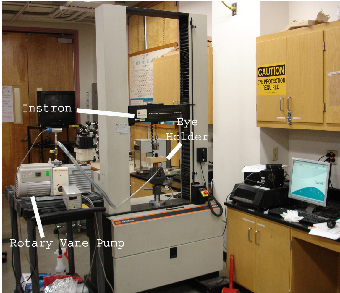
Figure 22. The adhesive force experimental setup. The rotary vane pump was positioned on the cart (far left), while the eye holder was clamped onto the universal testing machine.
